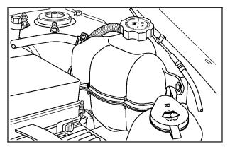
The surge tank is located on the driver's side of the engine compartment. See *Engine Compartment*Overview on page 5-12 for more information on location.
